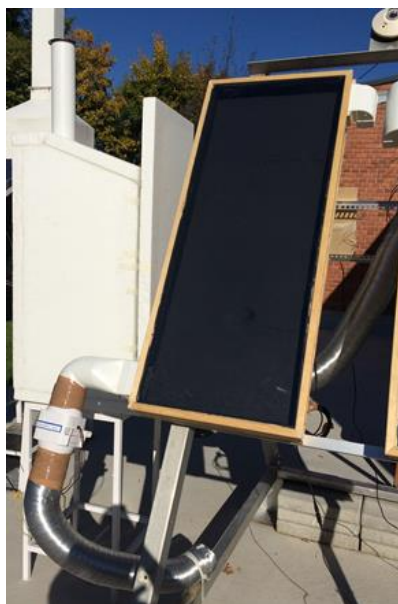
Fig. 1. Solar air heater at the laboratory of the Institute for Environmental Engineering System
