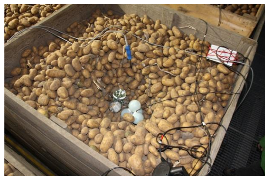
Fig 2. The ASL sensor placed in potatoes
